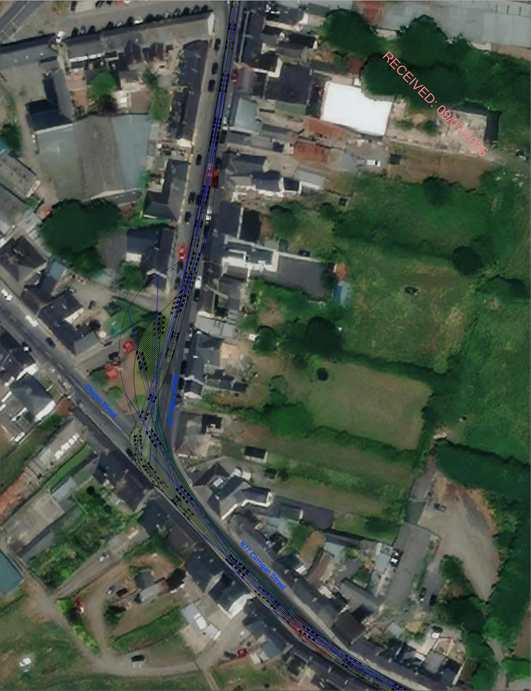
Figure 15-7 Location 1 - N77 Mary Street / N77 Carrigan Street / Chapel Street junction, autotrack assessment, blade extended artic
